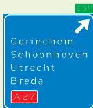
K4 High level motorway infor- mation sign showing lane in- structions for through traffic and exit panel showing inter- mediary destinations, with the motorway number and Eu- ropean route numbers
